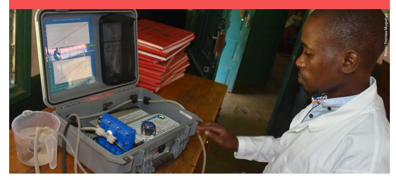
Aqua Research STREAM device operator observing the device while it produces hypochlorite disinfectant.
