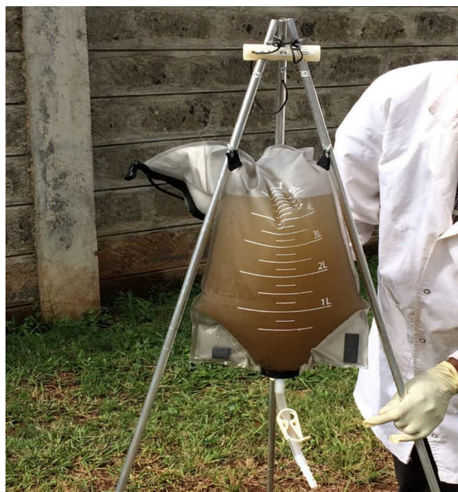
The BMFS captures traces of the poliovirus in wastewater. Photo: UW/Christine Fagnant-Sperati.
