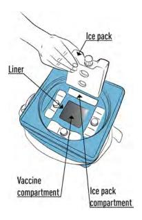
When the ice packs gradually warm from -25°C to 0°C, heat is drawn from ambient surroundings and from the liner.
