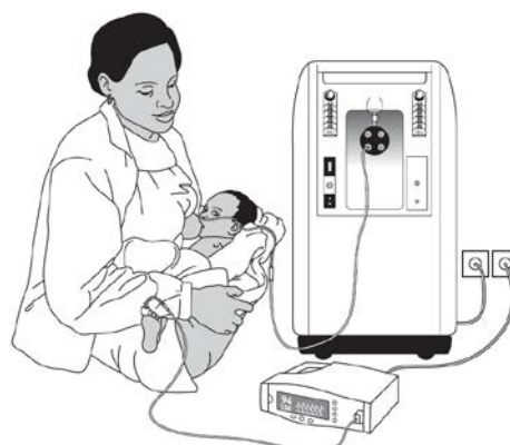
Setup of a pulse oximeter, oxygen concentrator, and connections to the patient. Image credit: PATH.
