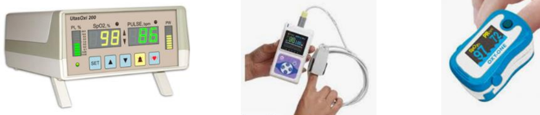
Figure 11. Pulse oximeters: tabletop, handheld, and fingertip, respectively.
