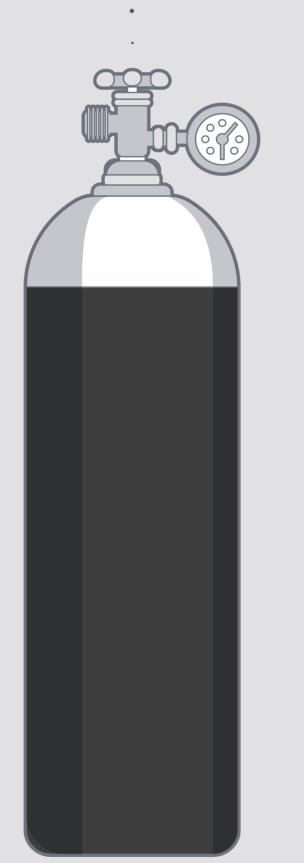
Do not use oil-based lubricant on the valves or other fittings of the gas cylinder.
