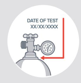
Please look for the next date of test, which is marked on a metal ring inserted between the valve and the neck of the cylinder, and if the date has expired, do not accept the cylinder for filling.
