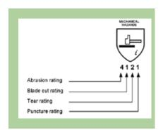
In this example the glove with a rating of 4 1 2 1 has excellent abrasion resistance (4), but a low cut resistance (1), good tear resistance (2) and a low puncture resistance (1).
