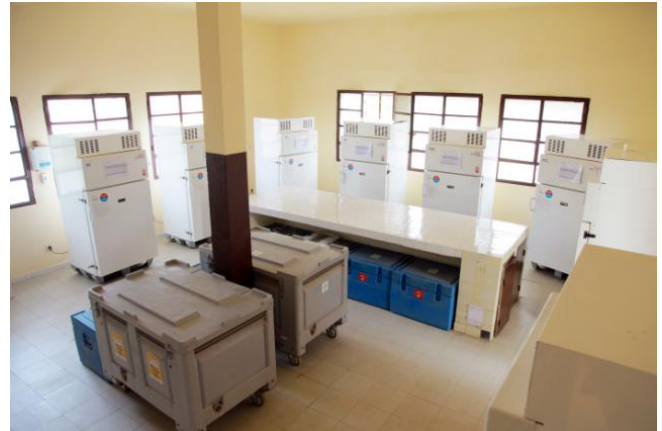
These direct-drive solar refrigerators by The Solar Chill Company were field-tested in Senegal. Photo: PATH
