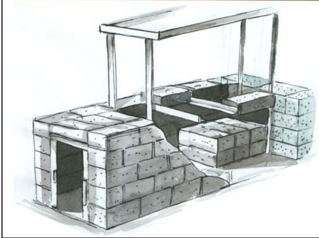
Figure 2.3.9 Adding refractory bricks around ash door and bridge
