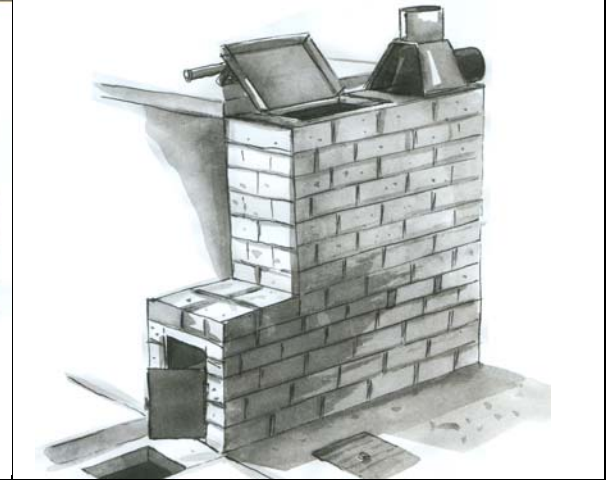
Figure 2.3.10 Finished incinerator masonry with loading door
